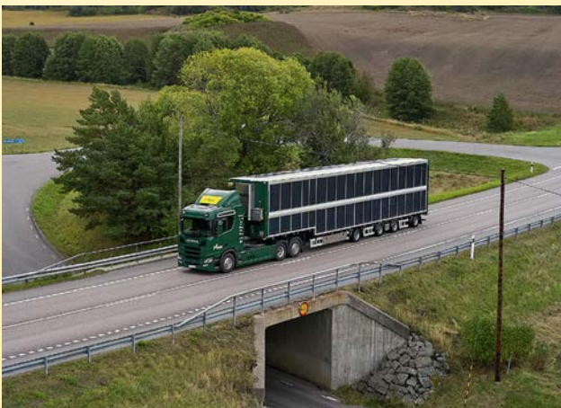
Scania’s solar-powered hybrid truck for which Midsummer is the exclusive supplier of solar panels.
